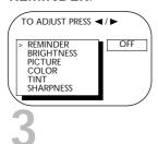
Press the REW(ind)/◀ button or the F.FWD/▶ button to select ON or OFF. Each press of the REW(ind)/◀ button or the F.FWD/▶ button turns REMINDER ON or OFF.
